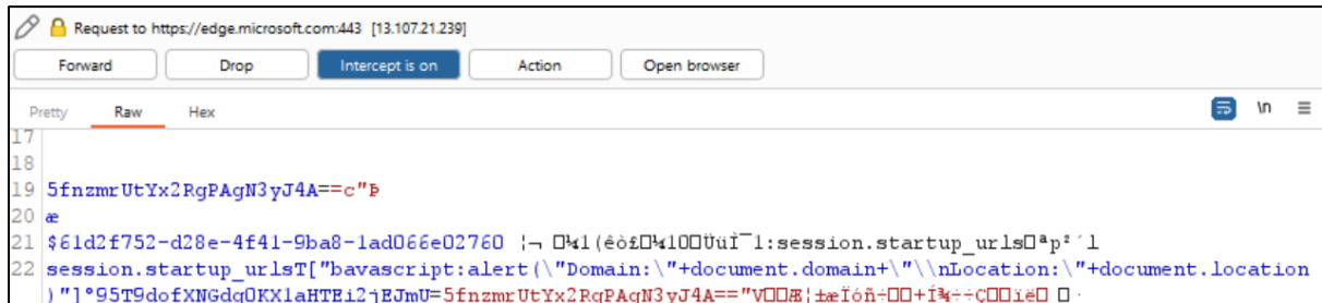
Figure 26: Sync request protobuf intercepted by a proxy, prior to modification.
