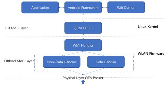
From the figure we can see that, Qualcomm WLAN firmware is not a *FULL MAC* firmware. The studies on Broadcom[1] and others show that, firmware of other vendors implement the full functions of the WLAN/WIFI stack. But Qualcomm is different, most of the MAC functions of WLAN/WIFI are implemented in the Linux Driver called QCACLD. The firmware of Qualcomm is much simpler. Thus leading to a smaller attacker surface in the firmware.
