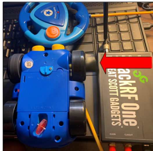
Figure 6: (Left): Capture of the 27.145MHz signal, (Right): Car's wheel rotating from replayed signal while control interface is off in background (arrow is pointing at blur which is a spinning piece of black tape)
