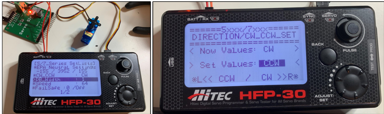
Figure 27: (Left): Servo test setup with Hitec HFP-30 programmer, (Right): Changing servo direction from CW to CCW.
