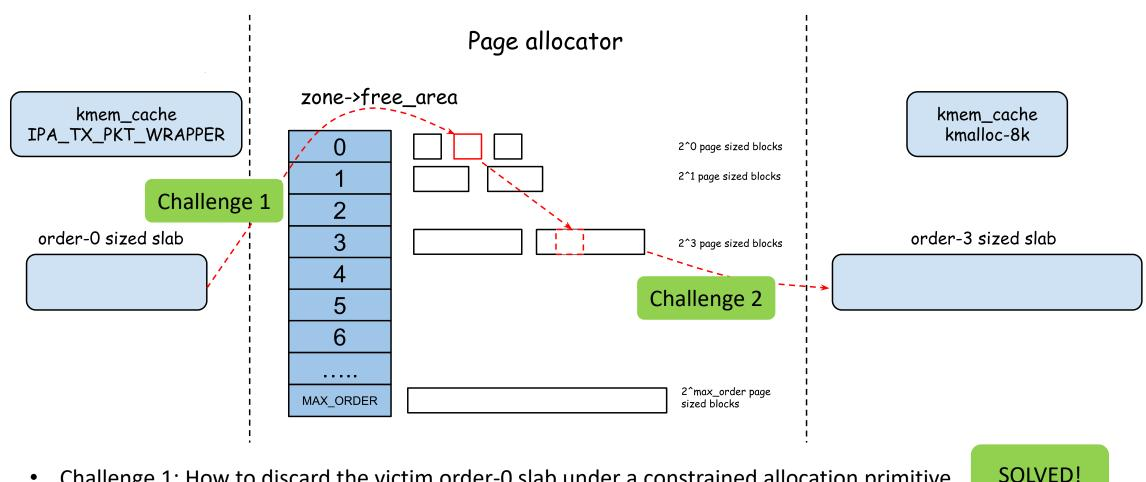
Challenge 1: How to discard the victim order-0 slab under a constrained allocation primitive
