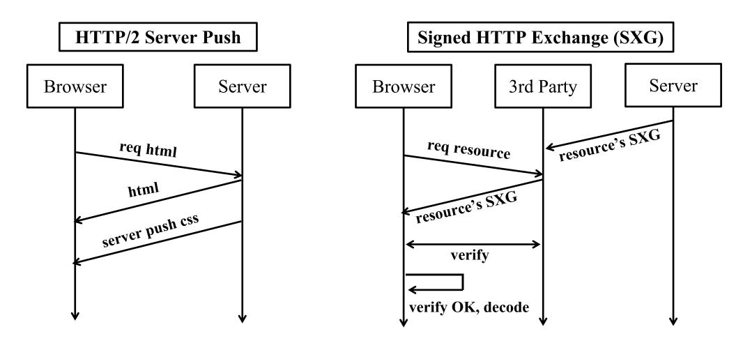
> Two server delivery mechanism designed to improve web performance
