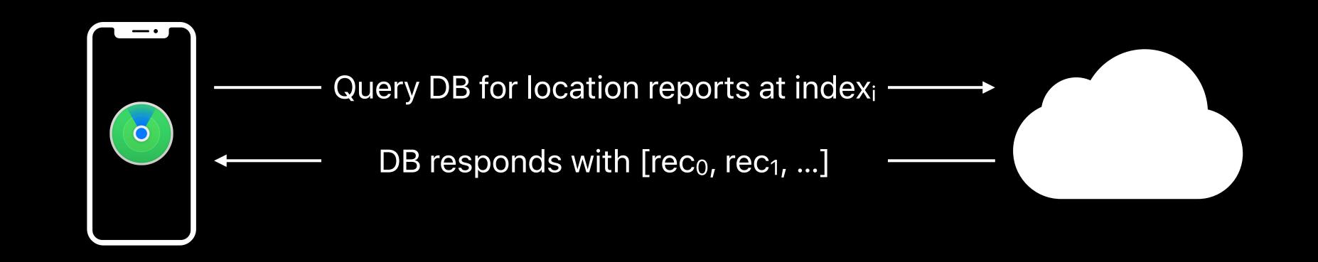
Retrieve  $d_i$  from iCloud Keychain Compute  $P_i = d_i \cdot G$  for lookup period i Compute lookup index<sub>i</sub> = Hash(P<sub>i</sub>) ECIES decrypt (pos<sub>i,0</sub>, time<sub>i,0</sub>) = D(d<sub>i</sub>, rec<sub>0</sub>)
