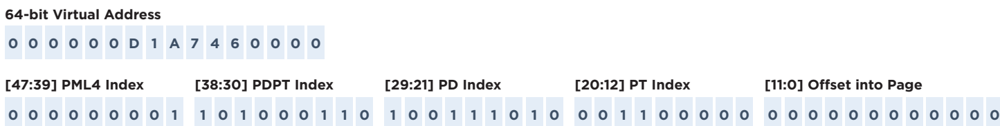
Figure 3: Intel 64-bit Virtual Address Translation.
