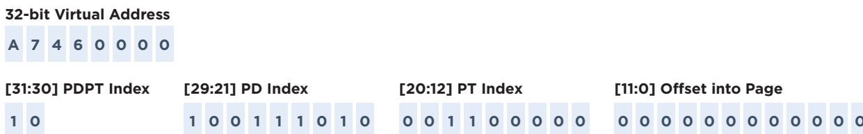
Figure 4: Intel 32-Bit Virtual Address Translation.
