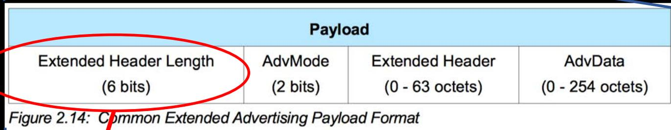
Example: ADV\_EXT\_IND Type, introduced on v5.0
