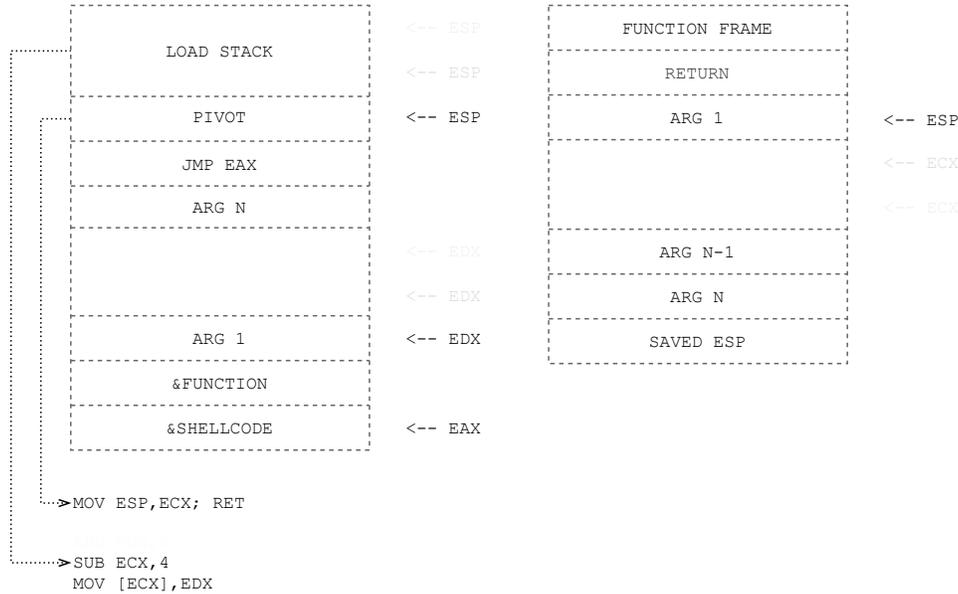
**Figure 3** Revised stack switching mechanism for the invocation of sensitive APIs guarded by Windows ROP mitigations.
