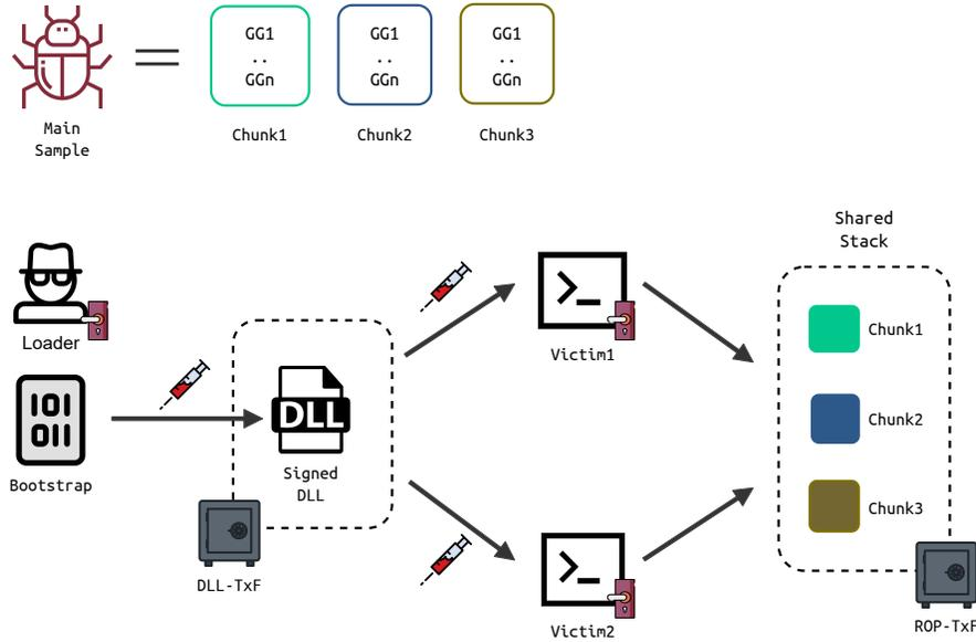
■ **Figure 1** Architecture of *Rope*. The payload is arranged in chunks that we place on a shared stack, the *ROP-TxF*, accessed by victim processes. We use another transacted file, the *DLL-TxF*, to deliver the bootstrap component. The loader component carries out the injection on each victim.
