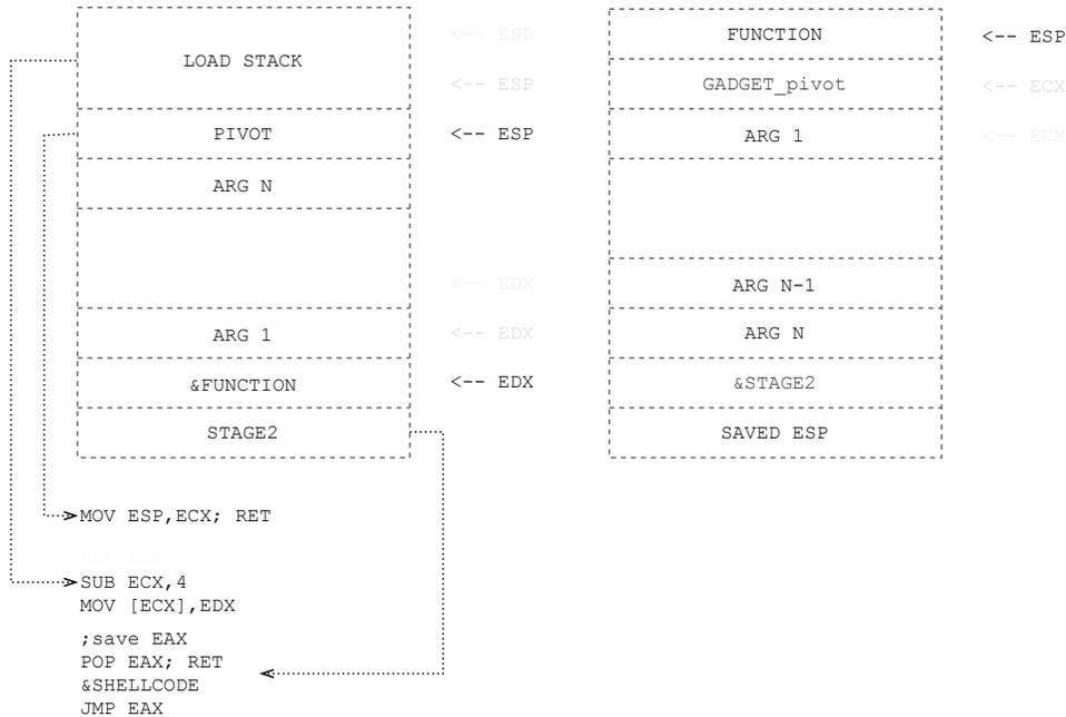
■ **Figure 2** Calling non-sensitive Windows APIs. On the left, the fragment of ROP chain for setting up a call. On the right, the native stack during the call. By `&SHELLCODE` we indicate the return address in the bootstrap component when implemented as shellcode. For the ROP-only variant of the bootstrap component we can follow the approach of [3] with custom stack-switching gadgets.
