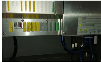
B) Inside the controller we learn about connectors and cables, which are exposed. The left side includes I/O and safety, whereas the right one leads to the main computer.
