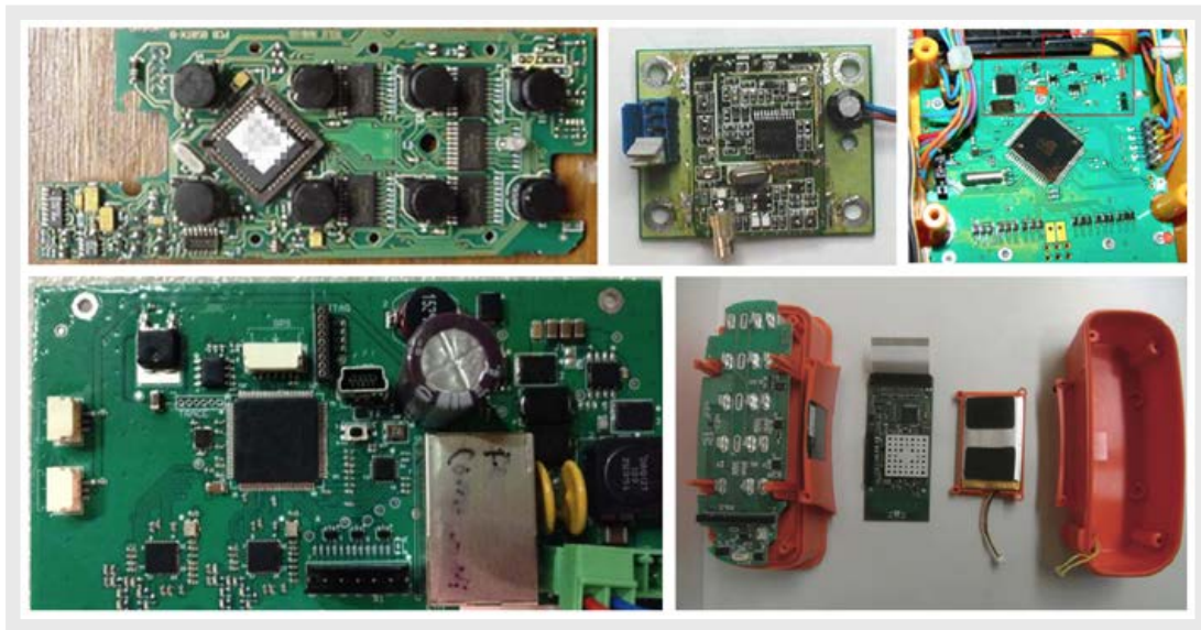
Figure 2. Evolution of the circuitry of industrial radio remote controllers (TX and RX) (main steps from 1997 to 2018), as seen in photos from user manuals and FCC documentation
