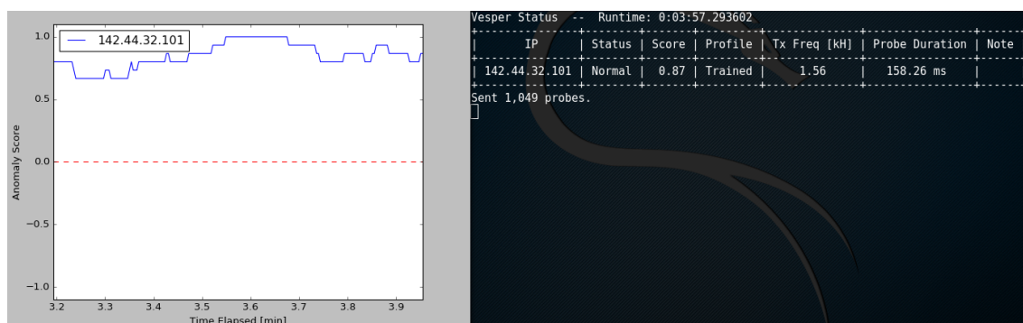
Figure 26: A screenshot of the tool in operation. Negative scores indicate abnormality.
