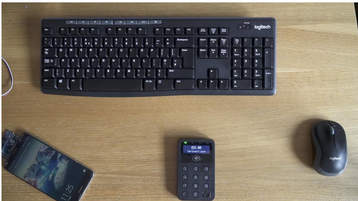
Figure 20. A contactless transaction of £31.00 with a consumer device. Screen must be active
