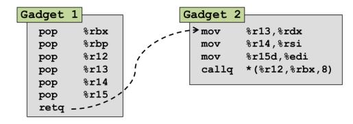
Figure 2: µROP chain from \_\_libc\_csu\_init
