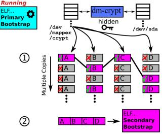
1 Extract shards of a new FLE image. Each shard was stored multiple times at pseudorandom locations to allow the error correction done here. Compare each shard copy's header against magic number:  $\sqrt{-}$  pass,  $\times =$  fail
