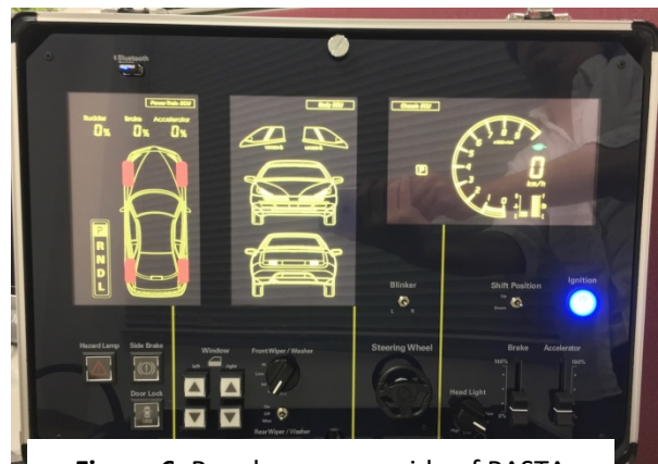
Figure 6. Panels on upper side of PASTA displaying vehicle status
