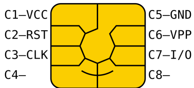
Figure 2: Smartcard pinout diagram
