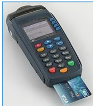
Figure 2 depicts a typical PoS terminal that's reading from an EMV chip card.
