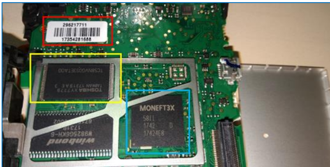
Figure 13 depicts our terminal's internal device ID in red, application processor in blue, and NAND Flash memory in yellow.
