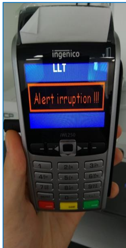
Figure 7 depicts a tampering alert on an Ingenico terminal's display.
