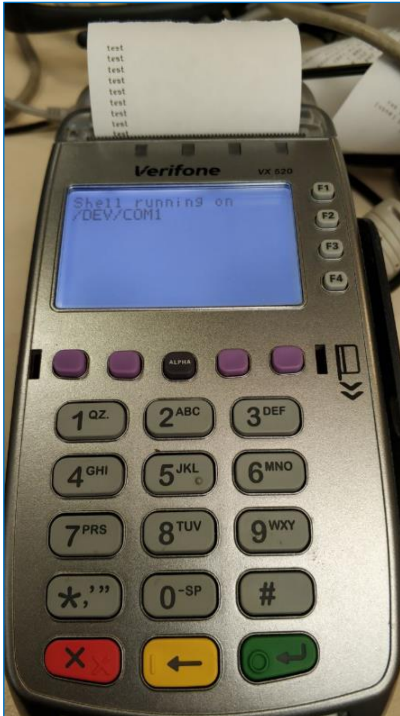
Figure 29 depicts the terminal's display while it's within the SHELL.OUT mode.
