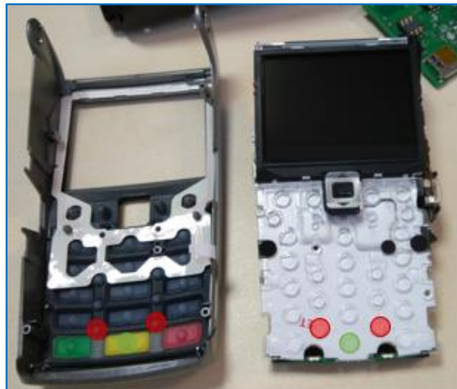
Figure 9 depicts the keyboard membrane with several key contacts highlighted in green and anti-tampering contacts highlighted in red.
