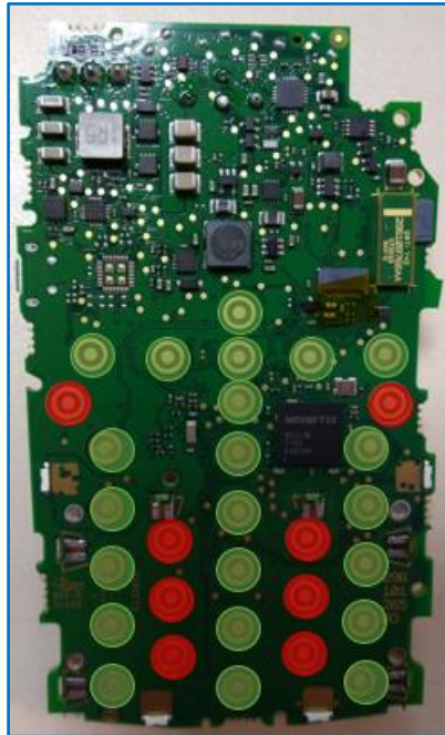
Figure 8 depicts the terminal's circuit board with key contact points highlighted in green and anti-tampering contact points highlighted in red.
