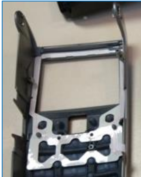
Figure 10 depicts the anti-drilling mesh on the top of the device.
