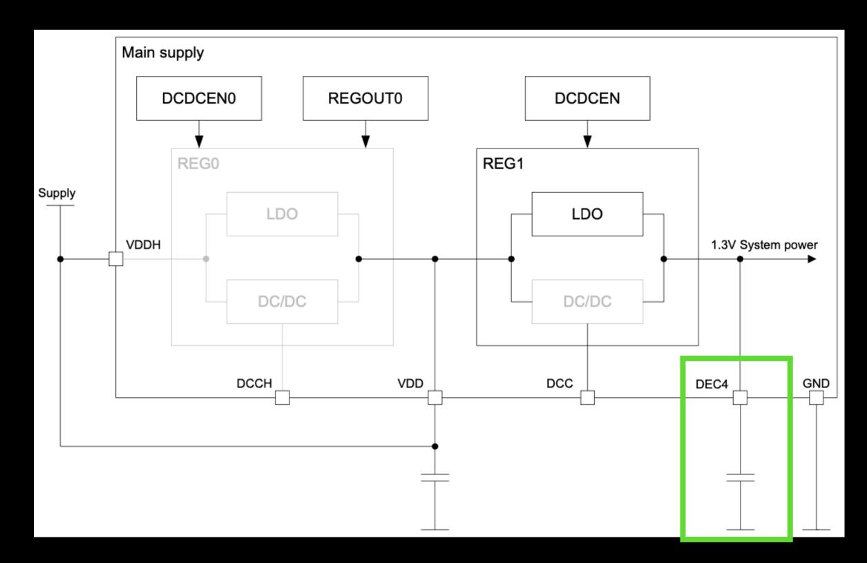
• DEC4 (1.2V-1.3V) is the power after the REG1 Stage, which supplies the
